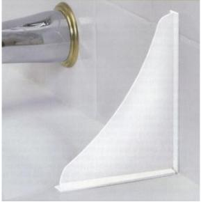
A lot of residents report water on the floor next to the bath tub. This is (most of the time) just water running off the tub. A sign that you have a problem like this is the increase in size (cracking) of the baseboard next to the tub. To prevent this you can install splash guards (see picture).
